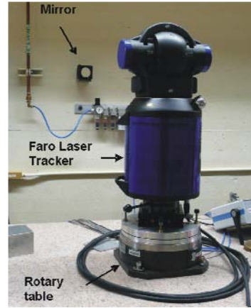
Fig 8: Faro laser tracker test setup
