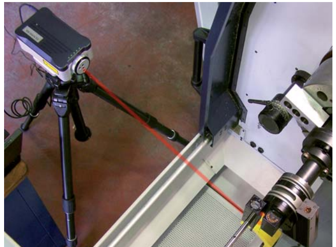
Calibration of a turning centre sub-spindle using the Renishaw RX-10 rotary calibrator
