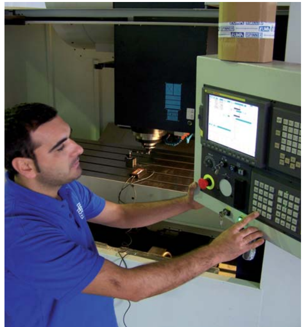
The QC10 ballbar takes only a few minutes to perform each test – Spinner use it to set up the control systems at the factory, then to help mechanically adjust out geometry errors caused by installation at a customer's site
