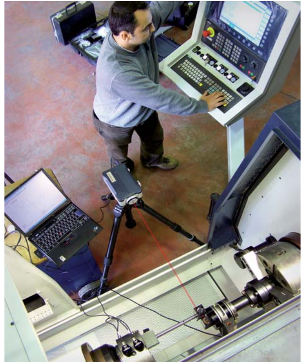
Mr Nurhan, Spinner’s Technology Manager, uses a Renishaw XL-80 laser and RX10 calibrator to test a sub-spindle on a Spinner CNC turning centre, guaranteeing the required repeatability
