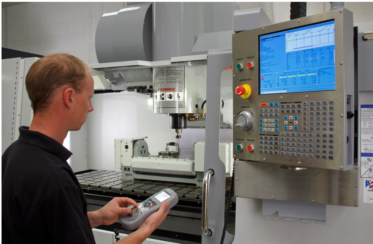
Performing a QC20-W ballbar test on a CNC machine tool
