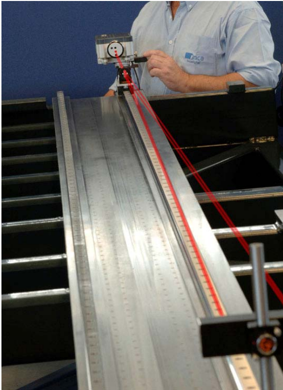
Machine main rails can be up to 11.5m – the XL-80 is more than capable of calibrating the full length of the table at the machine's top speed
