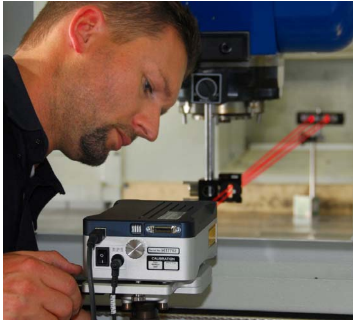
"LEDs on the top of the XL-80 make set up very straightforward, we can monitor the beam strength without going back and forth to the PC" comments Jürgen Emslander
