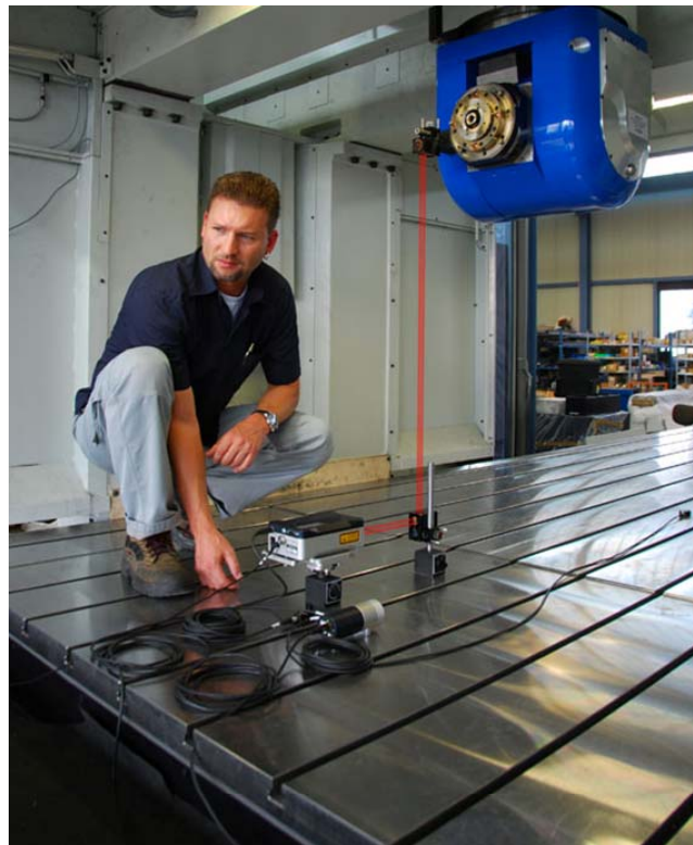
Jürgen Emslander can test accuracy with the compact XL-80 in many more positions, even inside machines like this Edel
