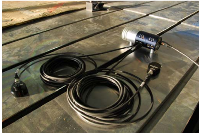
Sensors connected to the XC-80 compensation unit measure temperature and air pressure, allowing tests in any conditions
